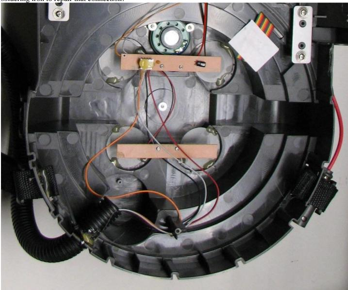
The bottom brown cyclotron board has two smaller separate red and black wires connecting it to the top brown board. We do not want this board, so cut the wires off near the top board. To make sure they do not accidentally short something, either cover the ends coming from the top board with electrical tape or cut them off flush with the top board (easier after the board is unscrewed from the posts holding it in place).
