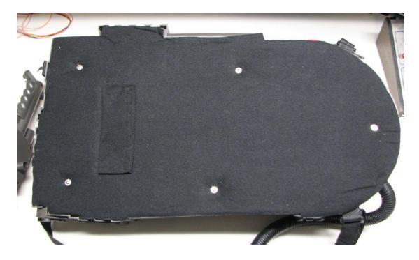
After re-installing the back cover, the screws can still be essentially hidden and only small cuts in the material above them allow easy access for the next time you want access in to the pack.
