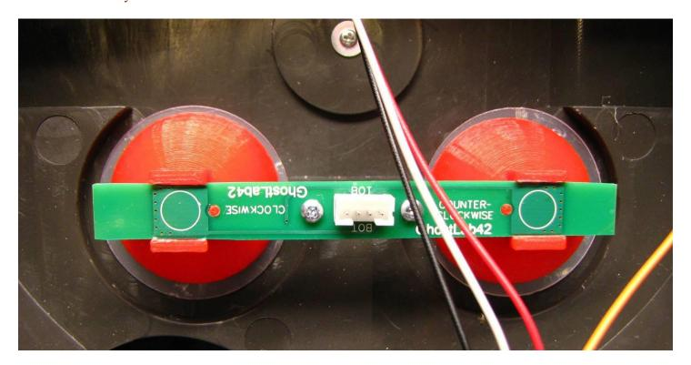
Orient the board with either the words CLOCKWISE or COUNTER-CLOCKWISE right side up, depending on which way you want the cyclotron firing order to progress when viewed from the outside facing the upright pack. Attach the new board with the reflectors to the two posts with the same two screws that were used to hold in the old brown cyclotron board.
