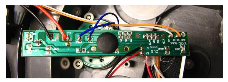
We now need to move the top brown board. We need this board for the sound and wand light, but we are going to mount the new board in its place so it must move up and out of the way. The wires do not allow it to move very far, so it just has to get out of the way!
