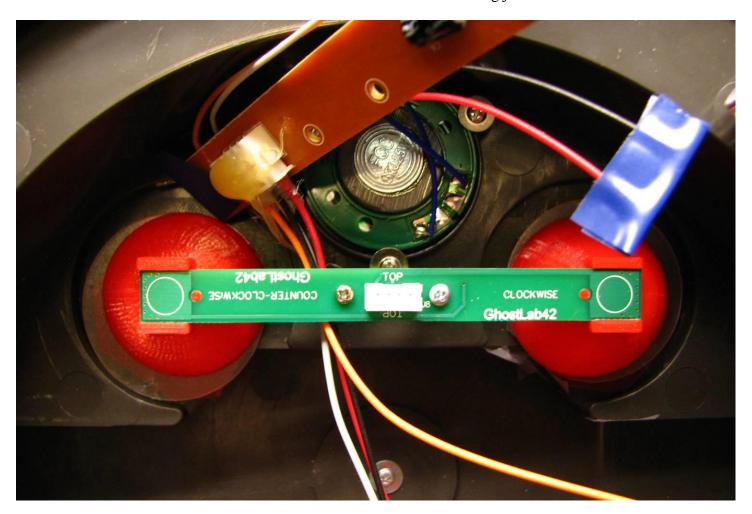
You can just use some electrical tape (or duct tape?) to hold the old brown board in place. We just don't want it flopping around but can't really move it anywhere useful without a lot of work.
