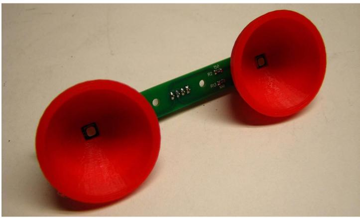
Orient the board with either the words CLOCKWISE or COUNTER-CLOCKWISE right-side up, depending on which way you want the cyclotron firing order to progress when viewed from the outside facing the upright pack. Attach the new board with the reflectors to the two posts with the same two screws that were used to hold in the old brown cyclotron board.
