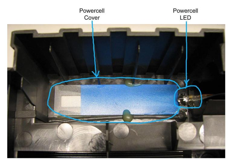
After the Cover and LED have been removed and the glue cleaned up (scraped off with small flat screwdriver):
