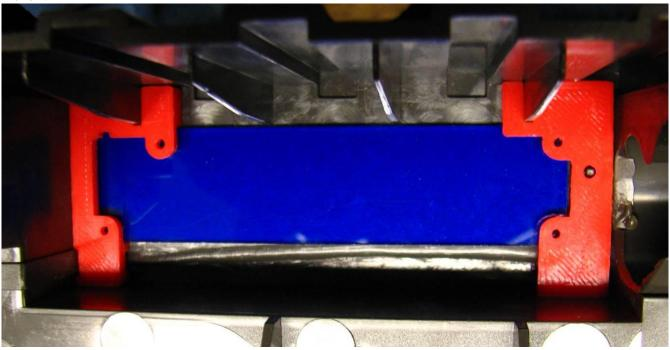
The top bracket (#7) is on the left side in the above picture and the bottom bracket (#6) is on the right-hand side. The brackets have many features in the bottom side (not visible in this picture) to hold the blue lens in place as well as go around various bumps, fins and support structures molded into the black shell. The blue plexiglass should be snug and practically held in place without needing any glue.
