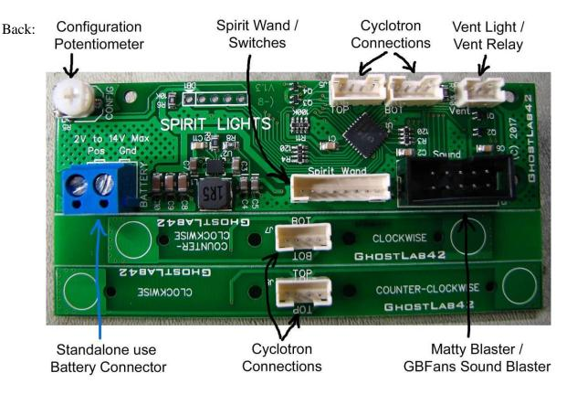
The Light Kit has a White configuration potentiometer on the back of the board to select between four main modes of operation:
